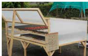
A direct model solar dryer (holds six trays), and protects drying vegetables from insects, dust and rain. Photos courtesy of Lisa Kitinoja
