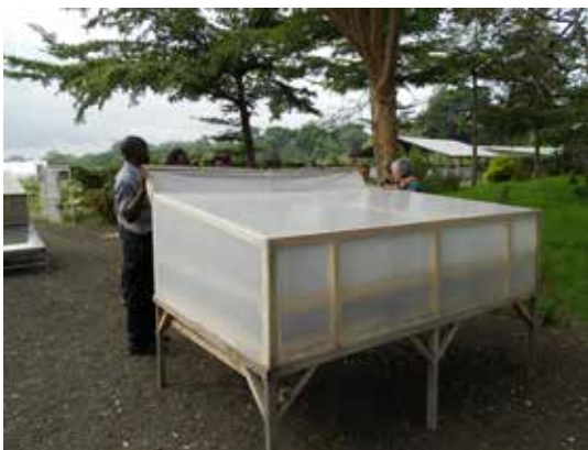
A direct model solar dryer (holds six trays), and protects drying vegetables from insects, dust and rain. Photos courtesy of Lisa Kitinoja
