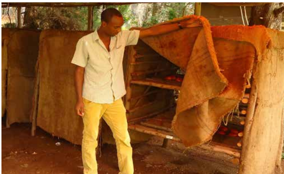
Desert cooler storage cabinet with shelves and a wet burlap cover. Photo by Esa Abiso for CRS
