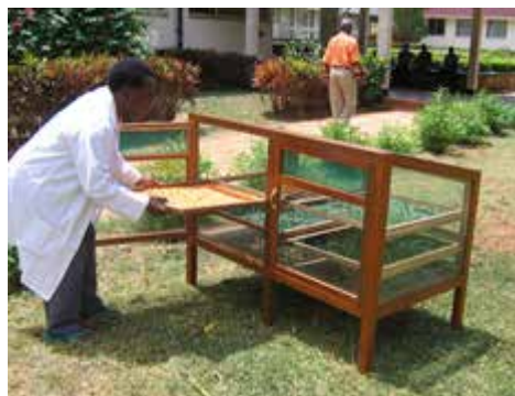
A solar drier in use in Tanzania (a direct model). Photo courtesy of Lisa Kitinoja/ Postharvest Education Foundation
